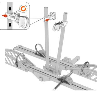
Install the adjustable Connecting Block (12) to the Middle Support Tube (10), then tighten the knob from the Connecting Block (12).
