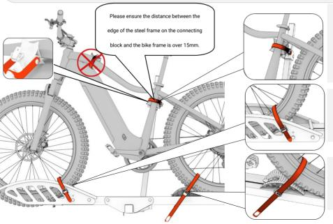
**Note:** Use the ratchet wheel strap to fix and tighten the seat tube, middle tube, or the position of the crossbar near the seat tube/middle tube of the bicycle.
