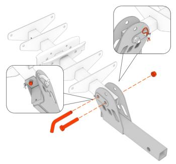
Align the Bottom Fixing Bracket(2) with the hole of the Rotating Group (1), insert the M16\*85 Outer Hexagon Bolt (3) into the hole at the bottom, and then screw on the M16 Lock Nut (4). Insert the 16 Bent Pin(13) and the  $\phi$ 3.8 Pin (15) at the same time, and use the M10 Short Hexagon Bolts (14) to screw into the Bottom Fixing Bracket (2) as shown in the figure to eliminate
