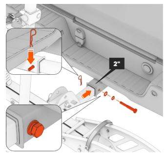
Align the holes of the folding tube with the holes on the vehicle's 2" hitch receiver, then connect the two parts as shown below. Place an M16 Shockproof Bolt (16), through the  $\phi$ 16 Spring Washer (17),  $\phi$ 16 Flat Washer (18) and the aligned holes. Screw the bolt in place by Monkey Wrench (Not included) and secure it
