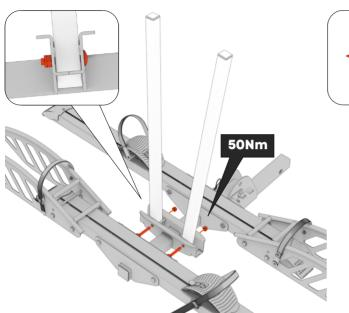
Insert the Middle Support Tube (10) into the base of the Bottom Fixing Bracket (2), then fix them with the M10\*60 Bolt (11) and the M10 Lock Nut (9).
