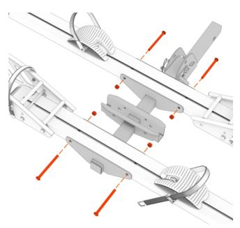
Place the components assembled in steps 2 above into the Bottom Fixing Bracket (2), align the holes, install 4pcs M10\*120 Outer Hexagon Bolt (8) and 4pcs M10 Lock Nut (9), and tighten the bolts.
