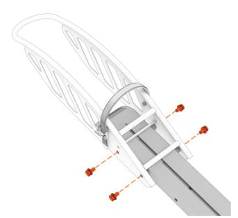
Align the holes from the **Front Wheel Holder (6)** and the **Beam Assembly (5)**. Then fix them with the **M10\*25 Outer Hex Bolt Kit**(7).
