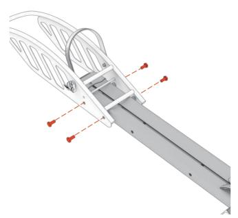
Put the holes of Front Wheel Mount (3) and Beam Assembly (1) aligned, install 4pcs-M10 Outer Hexagon Bolt (2) and tighten them.
