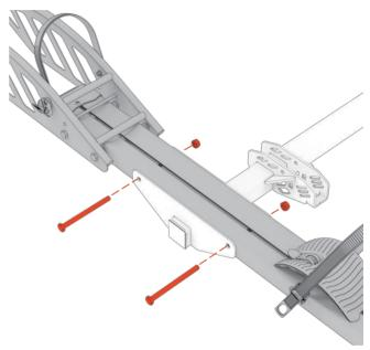
Place the components assembled in steps 1 above into the bottom fixing bracket assembly (6), align the holes, install 2pc Long Outer Hexagon Bolt (4) and 2pc M10 Lock Nut (5), and tighten the bolts.
