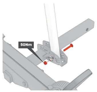
Insert the Support Rod (7) into the Bottom Fixing Bracket (6), align the holes, install M10 Low Square Neck Bolt (8) and M10 Lock Nut (5), and tighten them until the support rod does not move.
