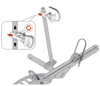
Insert Adjustable Support Assembly (9) into the Support Rod (7), and properly tighten the knob so that it does not slide down.
