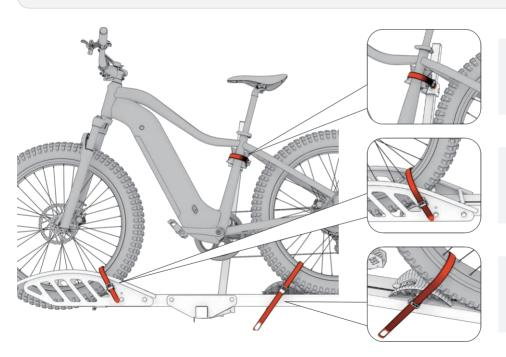
**Note:** Use the ratchet wheel strap to fix and tighten the seat tube or horizontal tube of the bicycle.
