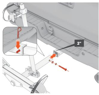
Align the holes of the folding tube with the holes on the vehicle's 2" hitch receiver, then connect the two parts as shown below. Place an M16 shockproof bolt (10), through the  $\phi$ 16 Spring Washer (11),  $\phi$ 16 Flat Washer (12) and the aligned holes. Secure the bolt in place with the  $\phi$ 3.8 Cotter Pin/Lock (13) making sure to place the pin through.
