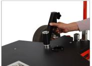
• Insert Seat Rod into Z-Bracket and lock it securely with locking knob.
