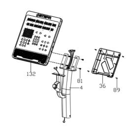
1. Hold the Console (132) and Upper Mast set carefully, connect the Console upper extension wire (118) to the Console lower extension wire (119).
