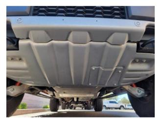
Step 2: On both the drivers side and passenger side, there is a bumper support strut, un bolt this from the bumper, and loosen at the frame side so that it can be rotated out of the way. Do this on both sides
