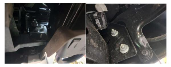
Step 6: Remove the rubber trim on top of the bumper, this can be done by squeezing the little triangle clips on the inside with pliers while pushing out. The white clips can be removed by pushing down on the retaining clip on the inside and pushing the whole white clip out of the black retainer. This is removed to trim for the light bar, or can be removed permanently, depending on your preference.
