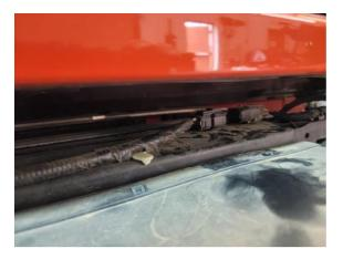
Step 7: Remove the 2 pictured factory bolts on each side. The inner bolt will require a spacer on each side. Align the light bar brackets with the two sets of holes and reinstall the factory bolts with the supplied spacers on the inside holes.
