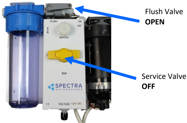
Valves in service position:
