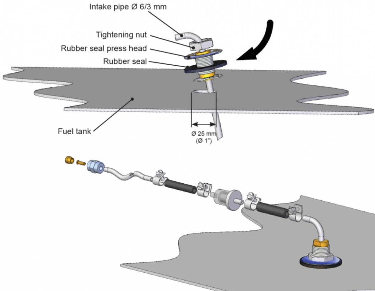
1. You will need to make a Ø 25 mm (1") hole in the upper surface of the fuel tank. Choose the location of the hole so that when the fuel tank tilts the end of the intake pipe will stay in the fuel even if the tank is not full. If the end of the intake pipe does not reach the fuel, the device will quickly choke on the air in the fuel system and that can cause malfunction to the system.
