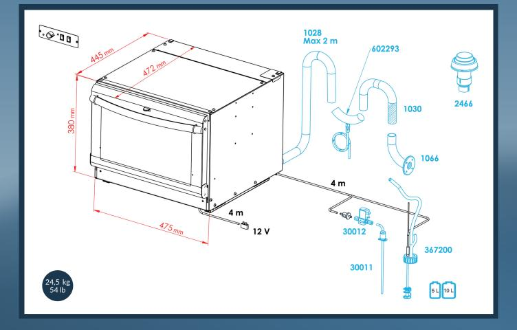
Accessories in black come with the standard package. Accessories in blue are additional/optional. The calculated values are measured in a reference measurement wall, which is constructed to represent a typical boat installation. The figures allow for 10 % reserve - yours may vary.
