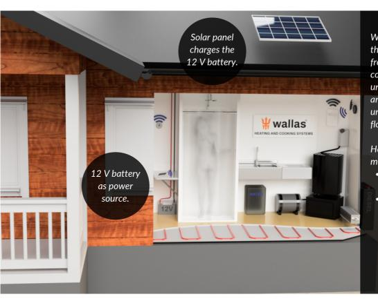
Water pump pushes the heat transfer fluid from the lowest pipe connection into the unit, hot water boiler and the heating pipes underneath the flooring.
