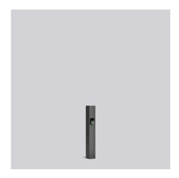
Charging column with square cross section. With EV charger to IEC 61851-1 Mode 3. For private applications. Luminaire tube made of corrosion resistant aluminium with pressure die-cast aluminium cover, seawater resistant powder-coated. With fully enclosed stainless steel mounting base. Stainless steel bracket and screws for EV charger unit. Elongated holes in base for easy bollard alignment. EV charger in integrated compartment with two type 2 charging sockets, lockable.
