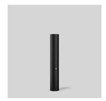
Luminaire tube made of corrosion-resistant aluminium profile, powder coated. Recessed stainless steel fixing plate. With C-track for junction box / fuse box behind the mast door. The robust stainless steel mounting base ensures long-term stability. Elongated holes in the base for subsequent and simple alignment of the luminaire, especially with asymmetrically wide distribution along a pathway.
