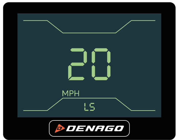
SETTING 2 - LS: Limited Speed. Max speed is 20mph, can be adjust to 25mph.
