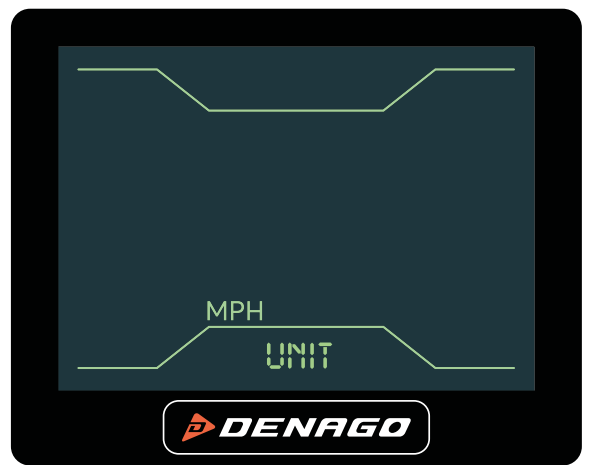
SETTING 4 - unit: this is the speed and distance setting MPH or KPH.
