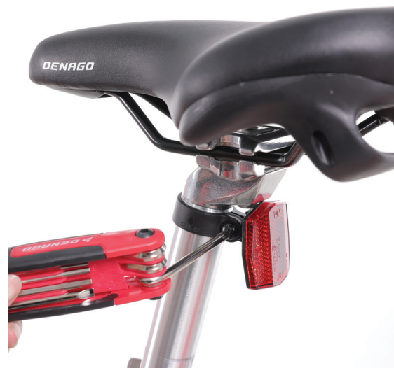
5. Take the rear reflector out of the bag and place it on the locking bolt of the seat tube.
