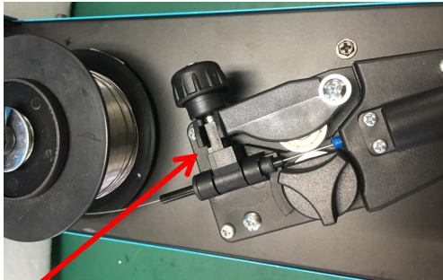
[7-9]Close down the top roller bracket and clip the pressure arm into place. Apply a medium amount of pressure to the drive roller
