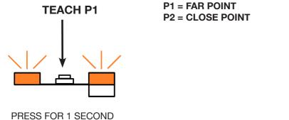
PRESS FOR 1 SECOND A, B ON, BLINKING BOTH 5 TIMES TO CONFIRM CORRECT TEACH
