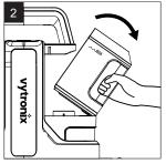
Remove the clean water tank. Note: pull the clean water tank at an angle of 30 degrees top to bottom.
