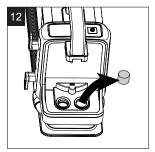
Remove small foam filter to clean by rinsing under the tap. Ensure this is fully dry before replacing and using in the appliance. TIP! Place on or near a radiator to dry.
