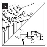
Re-install the empty clean water tank and power on, press the water-spray button to remove any excess water from the tank.
