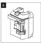
Empty the dirty water tank after every use or when the water level reaches the max fill line. The float inside will prevent suction if the tank is full.
