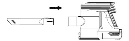
4. Attach the dusting nozzle to the extension tube or the main body works the same as the crevice nozzle.
