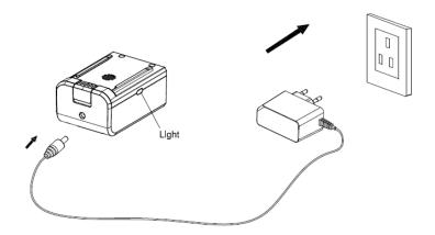
The battery can also be charged when it is housed in the main body directly. The three lights on the back of the body will indicate the charge level of the battery. When the battery is fully charged, the lights will always be **GREEN**.
