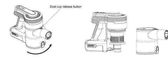
3. Over a waste bin, press the dust release button to open the bottom cover and expel any dust and debris. Wipe clean only, do not submerge in water.
