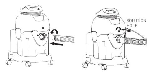
3. Connect the two parts of the aluminium tube together with the hose/handle.
