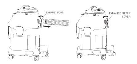
TOP TIP: After using as a wet vacuum or carpet washer, set up as above and use the blower function to quickly blow-dry the hose and remove any residual fluid before using the product for dry vacuuming.
