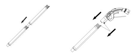
4. Connect the wet pick-up/wash head with the aluminium tube and connect all solution tubes/fittings.
