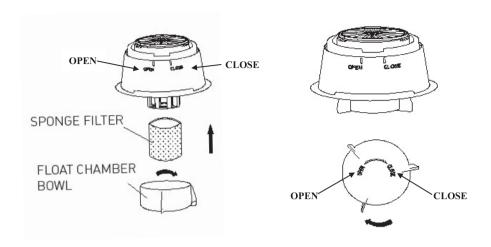
3. Clean the filters regularly and ensure filters are completely dry before reusing.
