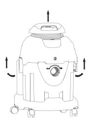
2. Disassemble float and filter housing and clean the HEPA and sponge filters per instructions on next page.
