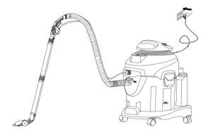
IMPORTANT: always turn on the main power button first, before switching on the pump when using as a carpet washer.
