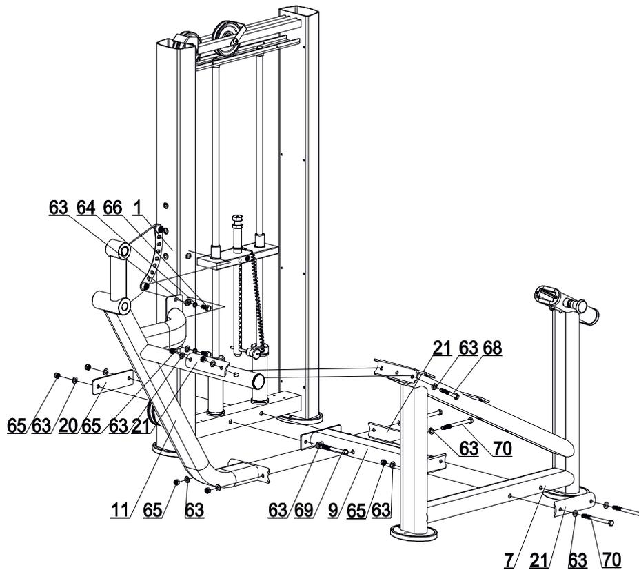
Assemble tower frame (1), main frame (7), connecting tube (9), curl support tube(11), fixing plate (20) and fixing plate (21), using flat washer(63), spring washer(64), lock nut hex M10(65), hex head bolt M10x25(66), hex head bolt M10x75(68), hex head bolt M10x100(69) and hex head bolt M10x125(70). Do not tighten the bolts and nuts at this step.
