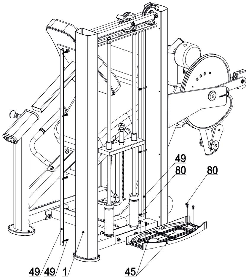
Install base cover (45) to tower frame (1) using pan head phillips bolts M6x15(80). Fix 2 side faces (49) in the tower frame (1) using 8 pan head Phillips bolt M6x15 (80), Using the right tools tighten bolts properly.
