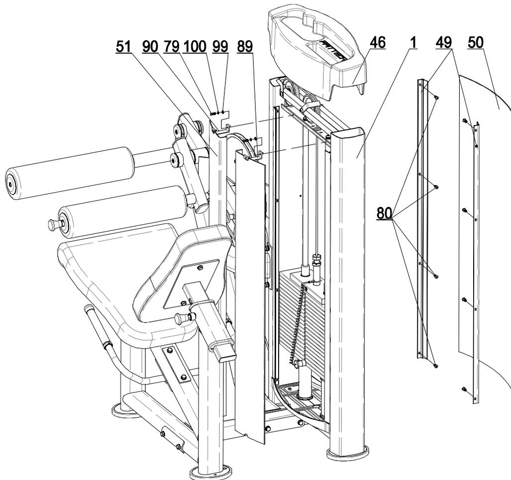
Fix 2 side faces (49) in the tower frame (1) using 8 pan head Phillips bolt M6x15 (80). Insert 2 front covers (51) and 1 back cover (50) in the tower frame (1). then fix the front covers (51) on the tower frame(1) using the left holder(89) and right holder(90), 2 pan head allen bolt M6x15(79), 2 flat washer(99), and 2 spring washer(100).
