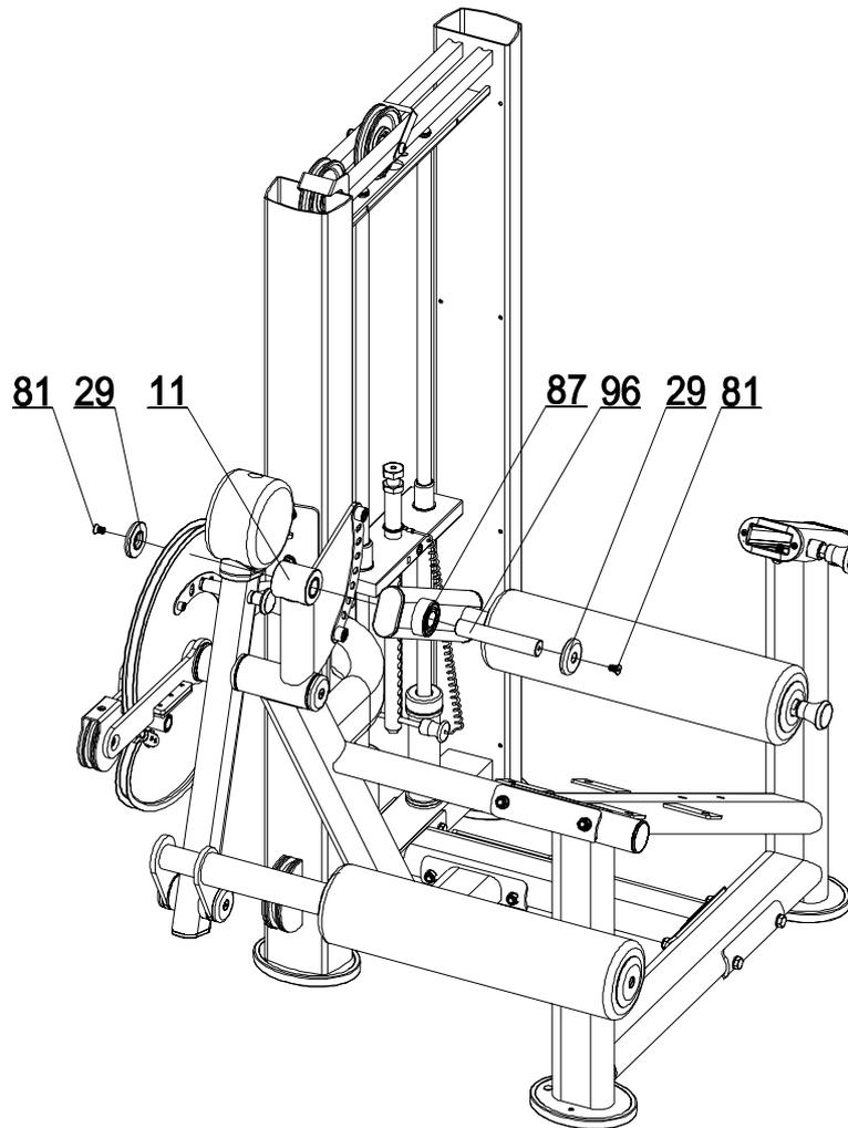
Insert foam Axis (96) into foam support(87),curl support tube (11), then fix using ending cap (29) and flat head, allen bolt (81).
