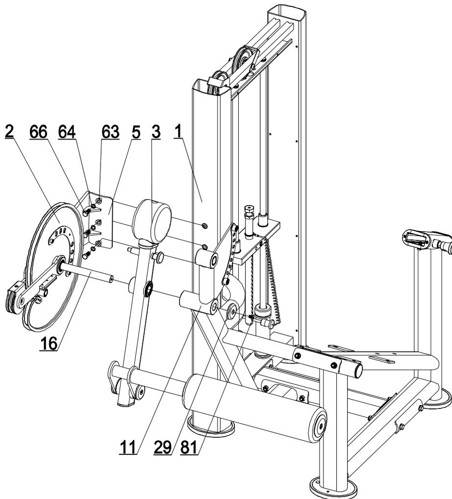
Install cam support (5) to tower frame (1), using flat washer (63), spring washer (64) and hex head bolt M10x25 (66). Do not tighten the bolts and nuts at this step.
