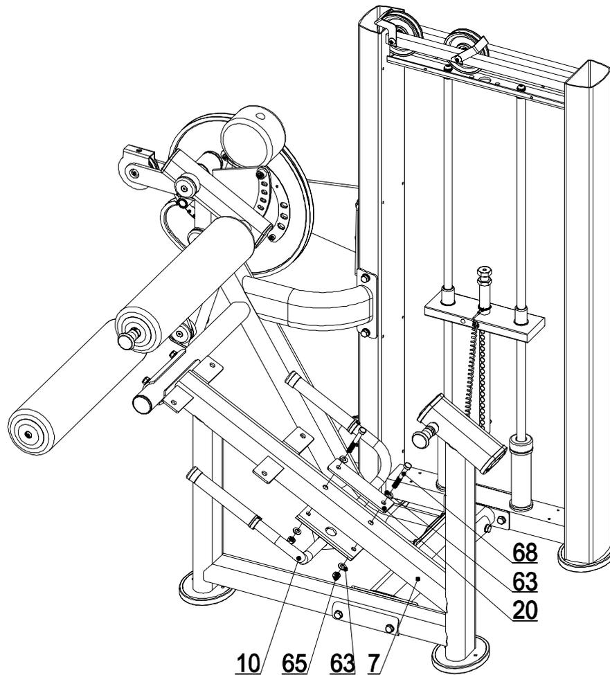
Install handle bar (10) and fixing plate (20) to main frame (7), using flat washer (63), lock nut hex M10 (65) and hex head bolt M10x75 (68).
