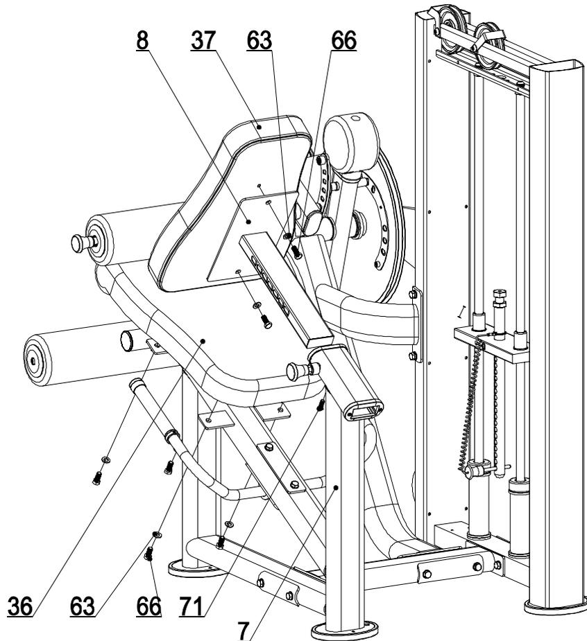
Fix back cushion (37) to the adjusting tube (8) using 2 flat washers(63) and 2 pan head Allen bolt M10x25(66), then remove hex head bolt M8x25(71) from main frame(7), install adjusting tube(8) to right position ,fixed the hex head bolt M8x25(71); Fix cushion (36) to main frame (7) using 4 flat washer (63) and 4 hex head bolt M10x25 (66). Use the right tool tighten the bolts.
