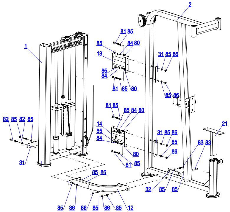
Assemble the tower frame(1) to the main frame(2) using connecting tube(12), connecting tube(13) and connecting tube(14). Fix it using 2 hex head bolt M10x125(83), 2 hex head bolt M10x100(82), 2 hex head bolt M10x25(80), 2 hex head bolt M10x75(81), 20 flat washer(85), 4 spring washer(84) and 8 lock nut hex M10(86), 3 fixing plate(21) and 1 fixing plate (32). Firstly adjust the position of the equipment and then using the right tools tighten bolts and nuts properly.
