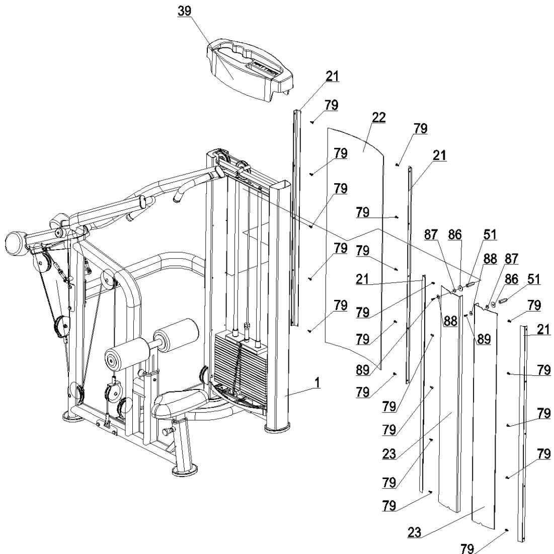
Fix 4 side faces(21) in the tower frame(1) using pan head Phillips bolt M6x15(79), 2 in the front and 2 in the back using the right tools tighten bolts properly. Insert 2 front covers (23) and 1 back cover(22) in the tower frame(1). Then fix the bolt(51) on the tower frame(1) using 2 pan head Phillips bolt M6x20(89), washer(86),washer(87),and big washer(88), and using the right tools tighten bolts properly. Put top cover(39) on the tower frame(1).
