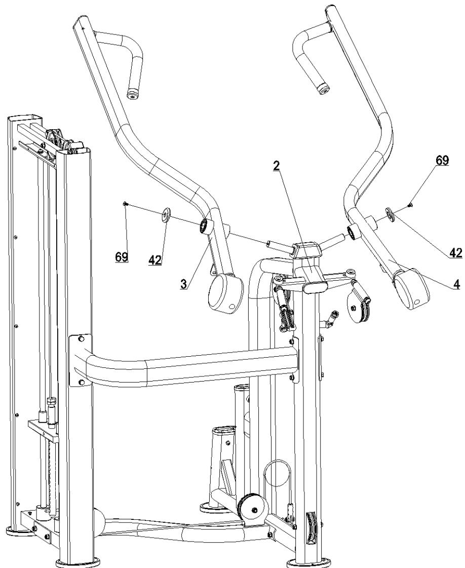
Connect left arm frame(3) and right arm frame(4) to main frame(2) using 2 ending cap(42) and 2 flat head Allen bolt M8x15(69) and using the right tools tighten bolts and nuts properly.
