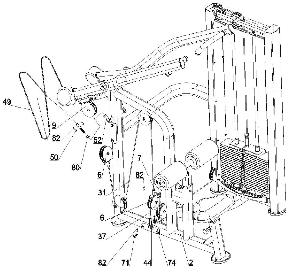
Fix nut hex M14(80) to the terminal(50), and fix terminal (50) to the joint bearing(52), tighten the nut hex M14(80)
