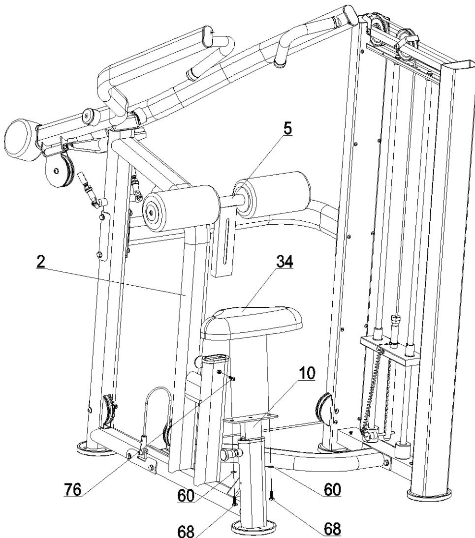
Remove hex head bolt M8x25 from the main frame(2), install cushion support(5) to main frame(2) using 1 hex head bolt M8x25. Fix seat cushion(34) to seat adjusting tube(10), using 2 hex head bolt M10x25(68) and 2 flat washer(60) and using the right tools tighten bolts properly.
