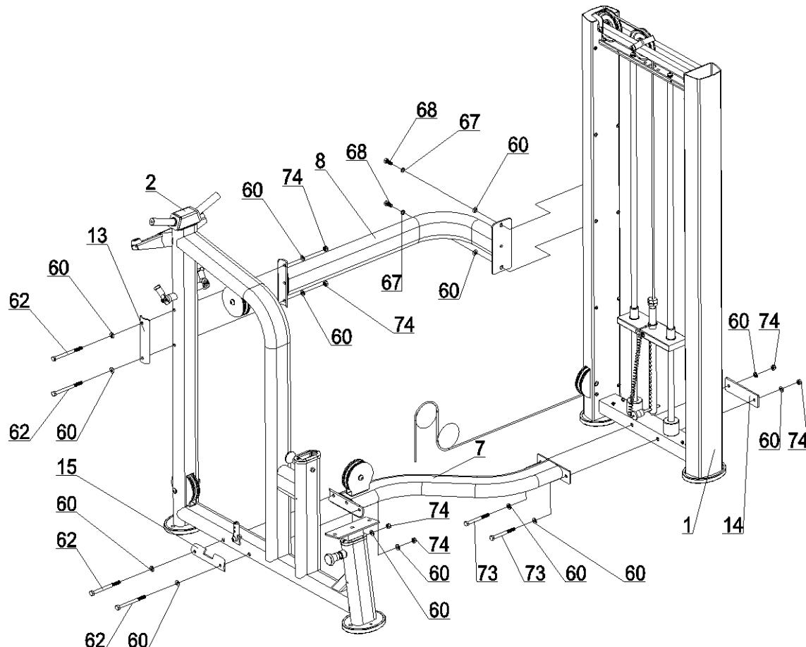
Assemble the tower frame(1) to the main frame(2) using connecting tube(7) and connecting tube(8). Fix it using 4 hex head bolt M10x125(62), 2 hex head Allen bolt M10x100(73), 2 hex head bolt M10x25(68), 14 flat washer(60), 2 spring washer(67), fixing plate(13), fixing plate(14), fixing plate(15) and 6 lock nut hex m10(74). Adjust the position of the equipment, and then use the right tools tighten bolts and nuts properly.
