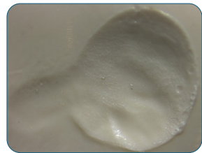
BioFlx after 800k Cycles of Wear Testing at 80 Newtons
