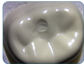
BioFlx after 800k Cycles of Wear Testing at 80 Newtons
