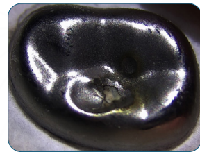
SSC after 400k Cycles of Wear Testing at 80 Newtons
