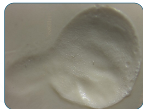
BioFlx after 800k Cycles of Wear Testing at 80 Newtons
