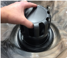
Pull Up to Remove Floater Assembly
