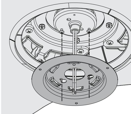
Feed the two single-pin connectors through the center hole of the upper switch housing, then wrap the keyhole slots around the screws and twist counterclockwise.
