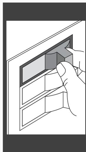
**English** To access the battery compartment, remove the battery door from the transmitter assembly. Install two AAA batteries, found in the remote control hardware bag, into the transmitter. Clean the battery contacts prior to installing the batteries.
