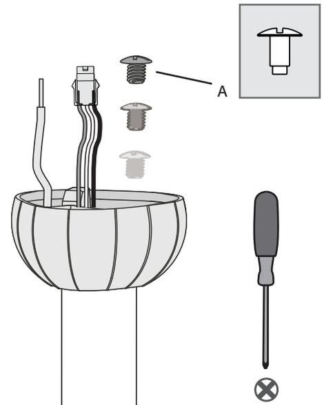
Insert the downrod ball screw (A) into the hole in the top of the downrod ball.
