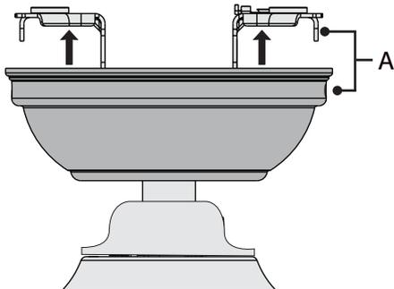
Lift the canopy into place so that the screw holes(A) are aligned.
