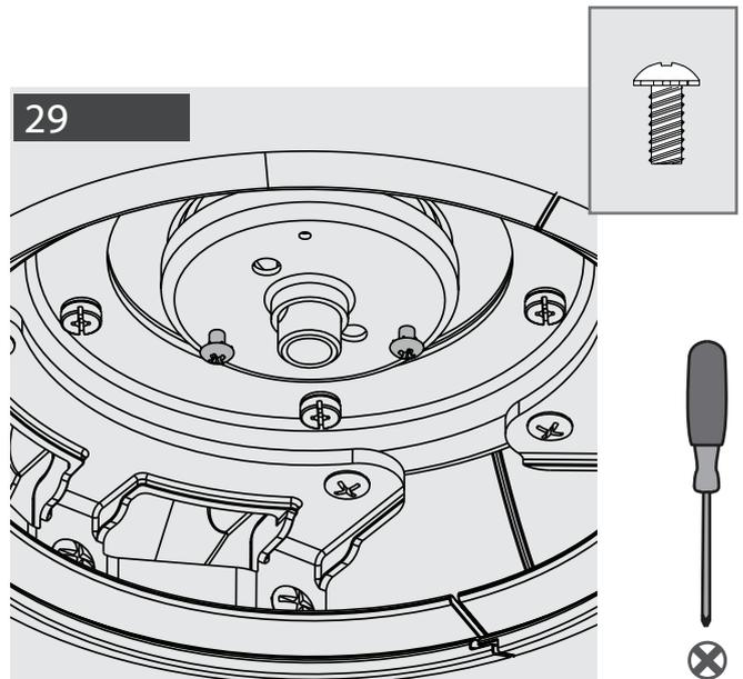
Screw two switch housing assembly screws, found in the ☐ hardware bag, halfway into the mounting plate on the bottom of the motor housing. It does not matter which two screw holes you choose.
