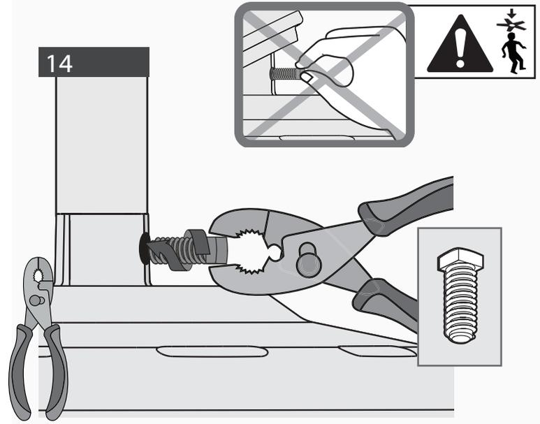
Tighten the setscrew with pliers. **DO NOT HAND TIGHTEN. FAN FALL HAZARD:** To prevent SERIOUS INJURY or DEATH, ALWAYS tighten setscrew with pliers. DO NOT hand tighten setscrew. CHECK the setscrew is tight using pliers each time you change fan direction.
