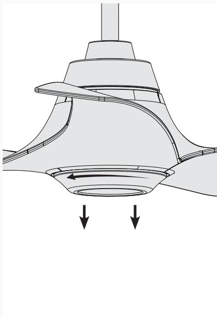
Carefully push up slightly and rotate the glass lens cap counterclockwise until it comes loose from the tabs and lower it from inside the LED assembly.
