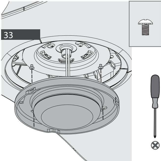
**33** Screw two light kit assembly screws from the
