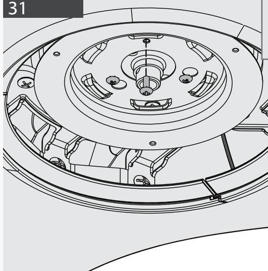
Insert the third screw found in the hardware bag
