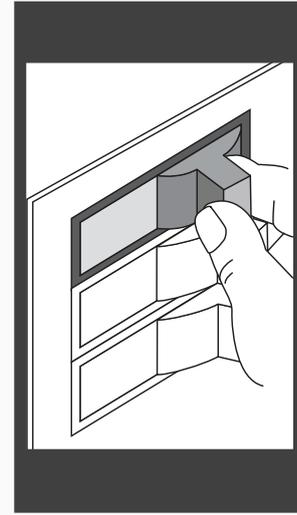
**English** Carefully lift the no-light cap up inside the LED assembly as far as it will go and rotate the cap clockwise until it is held tightly in place by the tabs.
