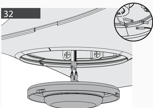
Connect the single-pin connectors from the LED assembly to the connectors from the fan.
