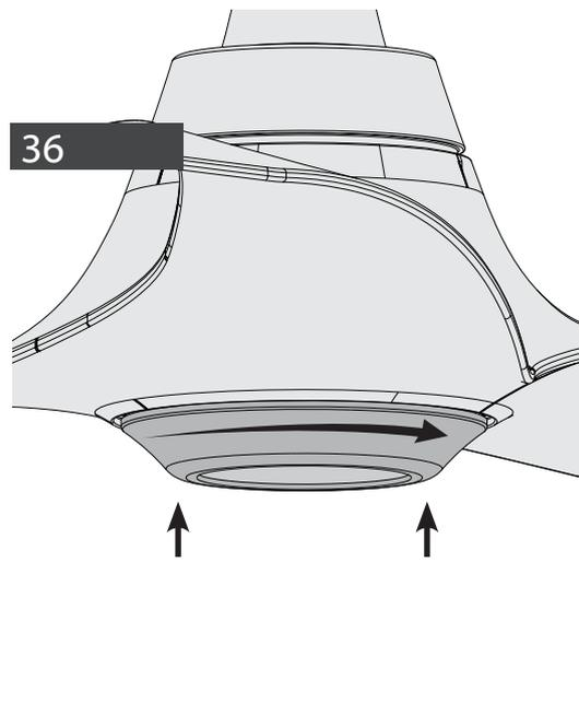
Carefully lift the glass lens cap up inside the LED assembly as far as it will go, then rotate the cap clockwise until it is held tightly in place by the tabs.
