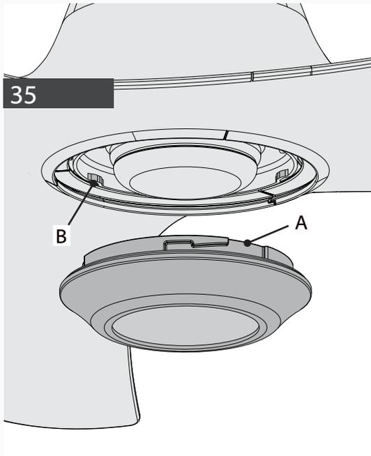
Position the notches (A) in the outer rim of the glass lens cap so they line up with the tabs (B) on the inside of the rim on the LED assembly.
