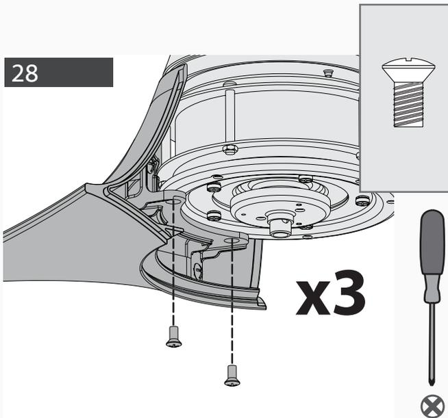
Attach each blade assembly to the motor housing as shown using two blade screws, found in the ☒ hardware bag. Securely tighten the screws after all three blades are attached.
