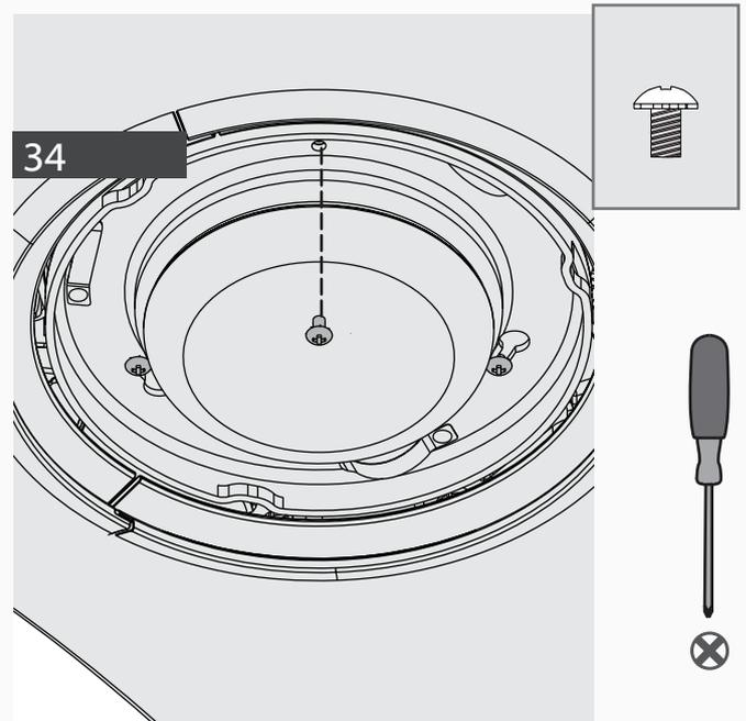
**34** Insert the third screw, found in the
