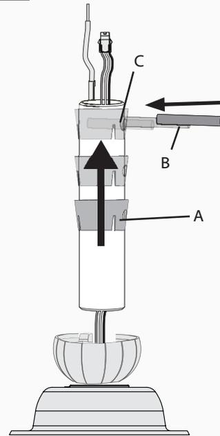
Slide the downrod sleeve (A) up the downrod. Insert the down rod pin (B) into the pin hole (C) on the top of the downrod.
