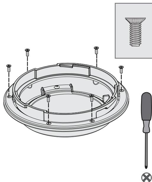
Uninstall the six screws around the outside of the glass lens cap. Remove the glass lens and set it aside for safe-keeping. Install the optional no-light cap using the same six screws. Tighten all six screws securely.
