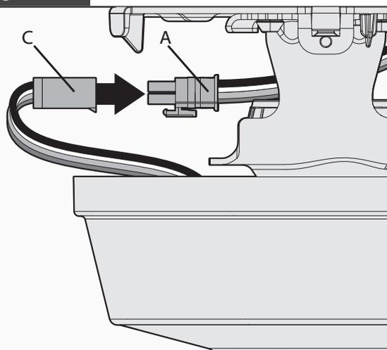
Connect wiring harness from canopy mount (A) to wiring harness from fan body (C).
