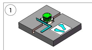
Place the concealed body in the desired position of the shower. Mark and drill (4) holes.
