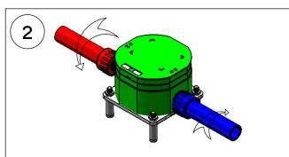
Connect the hot and cold supply pipes to the concealed body and check for any leaks.
