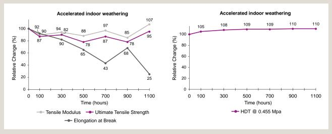
Note: For the indoor method, it is possible to infer that accelerated weathering times of 400 and 800 hours correspond to ca. 5 and 10 years of ageing in normal conditions, respectively.
