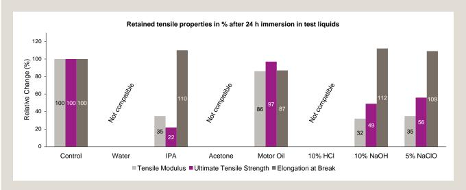
Note: after 7 days immersion, INFINAM® TI 5400 L retains excellent mechanical properties in motor oil, while the other liquids tested above are not compatible.
