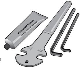
Popular mythology has it that the Wright Brothers (airplane inventors) originated left handed pedal threads to keep pedals from unscrewing while riding. It is a good practice to screw pedals in tightly after final fit adjustments have been made. Pedal threads - like most component threads on a bicycle should be lubricated lightly with grease.
