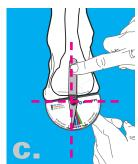
With FFMD in place, position the top flat surface of the Device (½-circle protractor) on ball of foot. Note angle indicated by the protractor. Repeat 3-times / foot to achieve a left & right forefoot tilt avg. Use this as your starting point for Cleat Wedge usage.
