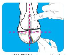
With FFMD in place, position the top flat surface of the Device (1/2-circle protractor portion) on the ball of the foot. Make a note of the angle indicated by the protractor. Repeat this procedure 3 times for each foot & average the numbers separately. Use this as your starting point. See reference charts found online at BikeFit.com
