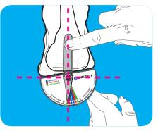
With FFMD in place, position the top C. flat surface of the Device (1/2-circle protractor portion) on the ball of the foot. Make a note of the angle indicated by the protractor. Repeat this procedure 3 times for each foot & average the numbers separately. Use this as your starting point. See reference charts found online at BikeFit.com
