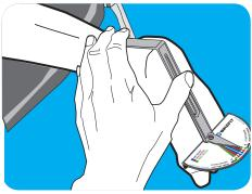
Your BikeFit Pro will place the Forefoot Measuring Device (FFMD) on the bottom of each foot pushing the handle against the heel so the vertical portion is aligned dividing the heel in two equal halves. The FFMD can be purchased separately at www.BikeFit.com.
