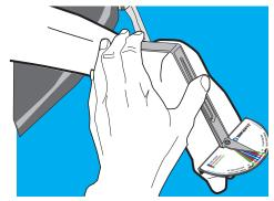
Your BikeFit Pro will place the Forefoot Measuring Device (FFMD) on the bottom of each foot pushing the handle against the heel so the vertical portion is aligned dividing the heel in two equal halves. The FFMD can be purchased separately at www. BikeFit.com.
