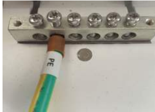
Figure 4.10 Grounding Terminal on Heat-Sink
