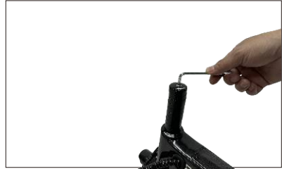
02 Loosen the head tube screws
