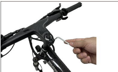
05 Tighten the screws on the side of the head tube
