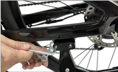
03 Use the matching tool to tighten the screws
