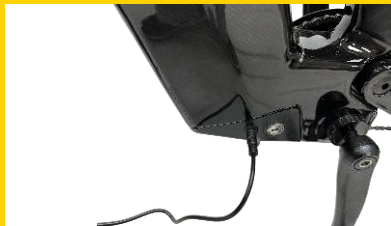
A. Recharge the battery on E-bike directly
