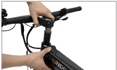
04 Ensure that the handlebars are evenly placed
