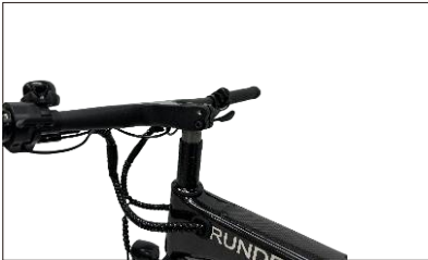
03 Place the handlebar into the head tube
