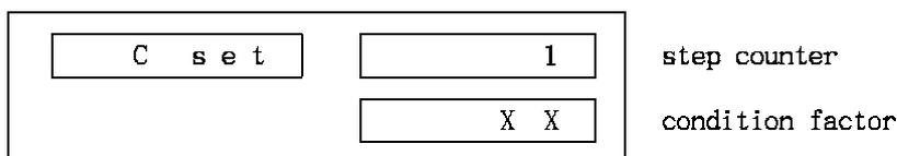
Press **STORE** key to go to next step and after finishing 4 times entering, display shows "End" message.
