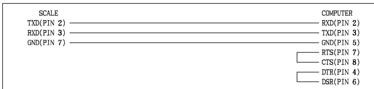
A.2.2 THE WIRE CONNECTIONS OF THE D-SUB 25 PIN CONNECTOR OF A COMPUTER SIDE
