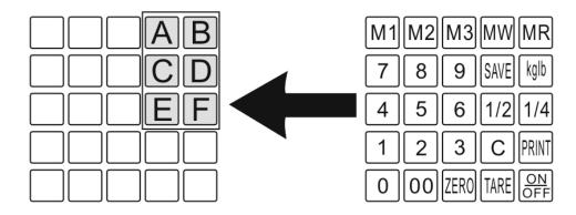
7. Press the "C" and the scale will show the version, count up, and then go to the weigh mode.
