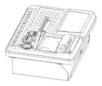
⚠ When closing the cover, Press the center of printer cover firmly to prevent paper miss-loading
