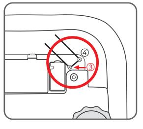
Input the Sealing Wire to the hole of Sealing Bolt ③ ④※ ③ CALIBRATION BOLT
