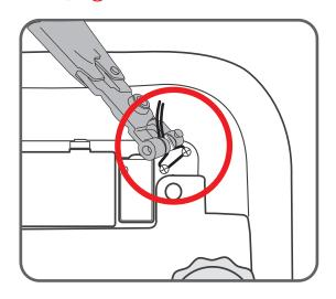
O3 Press strongly Al Sealing bar with Sealing Wrench
