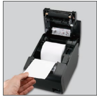
Easy paper loading & Jam Free/Apply auto cutter
