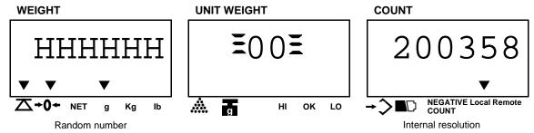
Press SET key to check the current internal resolution. Display shows as below:
