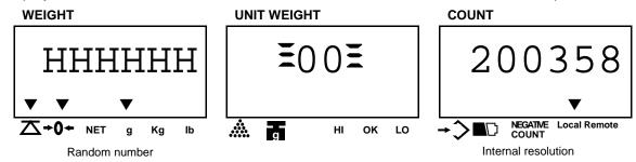
1.2 If display shows as below, it means the scale has been calibrated before.
