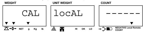
Then press **ENTER** key for determination and enter into calibration mode.
