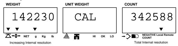
Weight window shows the increasing internal resolution, Count display window shows the total internal resolution which equals to original one and the increasing value.
