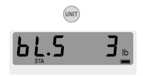
■Click [UNIT] to increase the brightness, the minimum brightness is 0 (without backlight), and the maximum brightness is 9.
