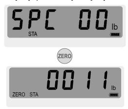
■Click [UNIT] key to modify Spec 00. The display will show SPC 00, and then press the [ZERO] to enter the power saving mode.
