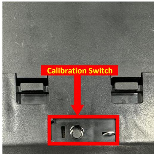
3. While holding the **ZÉRO** button, hit **UNIT** **TARE** **TARE** to enter the calibration mode. The display will show the default calibration weight.
