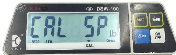
6. Place the calibration weight and press the **ZÉRO** button.
