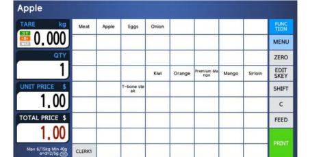
4 Place an item on the platter and press the V1 key.
