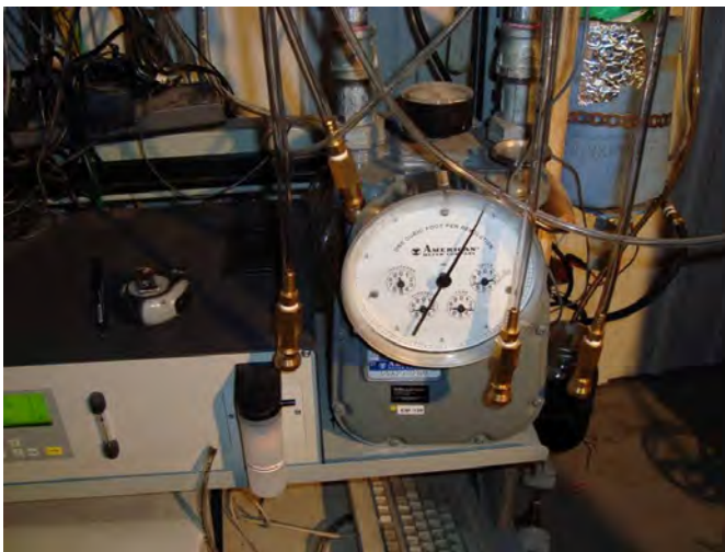
Picture 8: Reference dry gas meter
