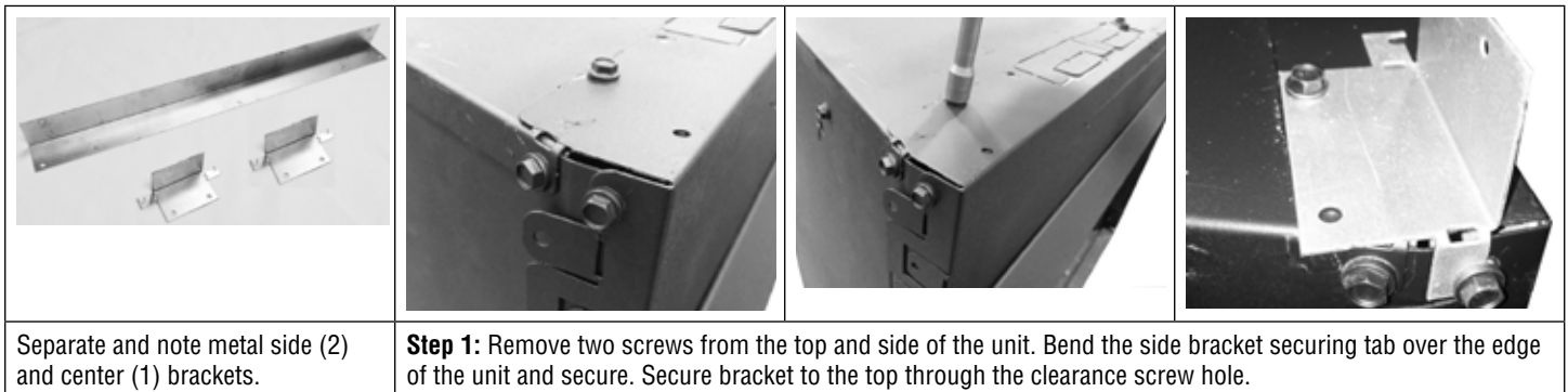
Figure 8 - Non-Combustible Front Fireboard Standoff
