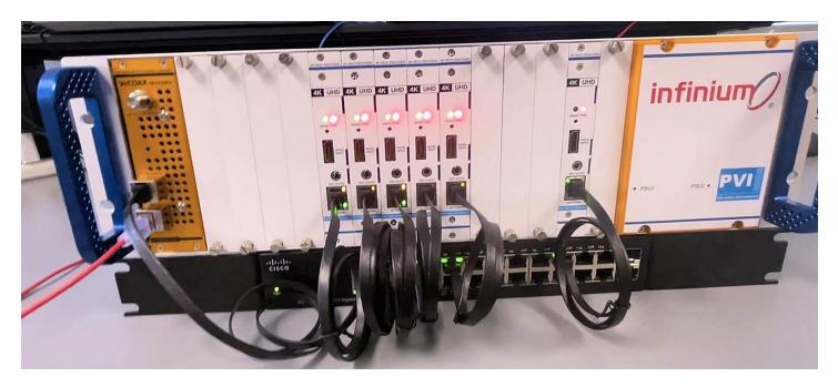
In this example the RED COLOR cable goes to the computer to control the IPMOD Module separately
