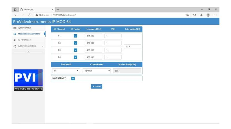
RF ENABLE: turn on/off the output of this frequency on the coaxial spectrum
