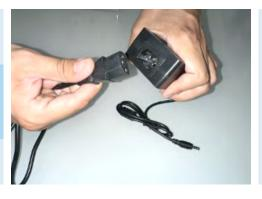
Connect power supply to the LSG, between the timer dial and indicator light.
