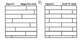
Continue nailing and gluing 2-3 rows at a time in this manner across the room. Avoid creating "H" patterns (where an end joint is adjacent to another end joint in the second to last row installed). Use cut ends to start the subsequent row, discarding any pieces shorter than 8".
