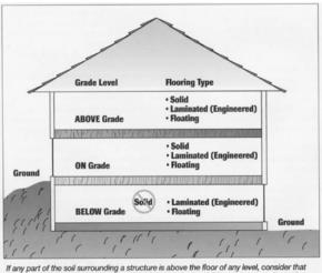
If any part of the soil surrounding a structure is above the floor of any level, consider that level below-grade. This includes walk-out basements. In addition, the surrounding soil should be sloped away from the structure with at least 6 inches of fall over the first 10 feet
